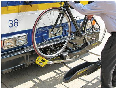
Lift bike into the rack, fitting the front wheel into the frame facing the same side as the yellow support arm.
