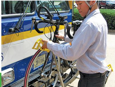
Pull yellow support arm up and over front tire as close to the frame as possible. The support arm should rest securely on the front tire ONLY, not on the bike's frame.
