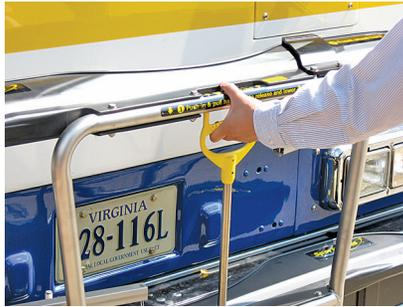
Lower the rack using the yellow release handle. The first bike in the rack should be loaded in the position closest to the bus.
