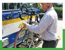
Pull yellow support arm up and over front tire as close to the frame as possible. The support arm should rest securely on the front tire ONLY, not on the bike's frame.
