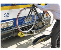
Lift bike into the rack, fitting the front wheel into the frame facing the same side as the yellow support arm.
