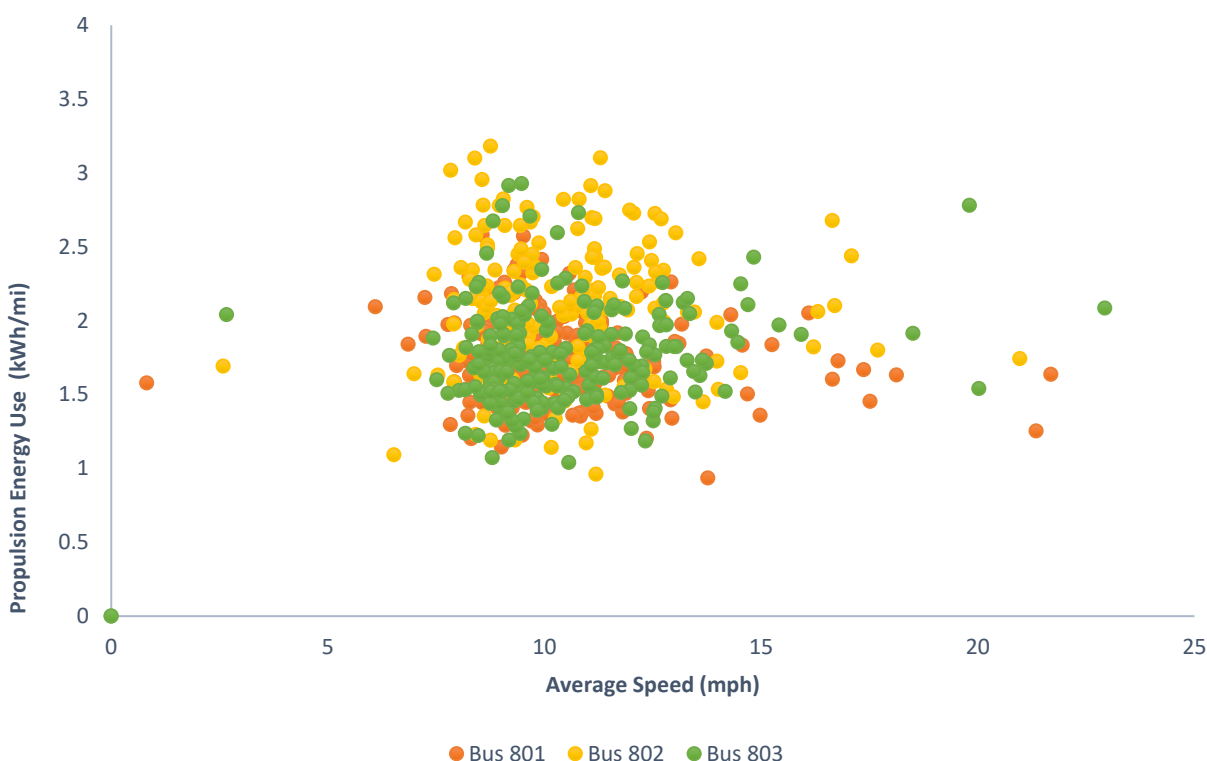
Figure 2. New Flyer 40-foot BEB Average Propulsion Energy Use versus Average Speed
